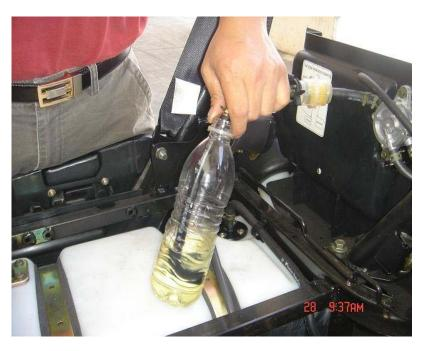
STEP 4: PLACE THE HOSE FROM THE FUEL TANK INTO A CONTAINER THAT HAS GAS IN IT.
