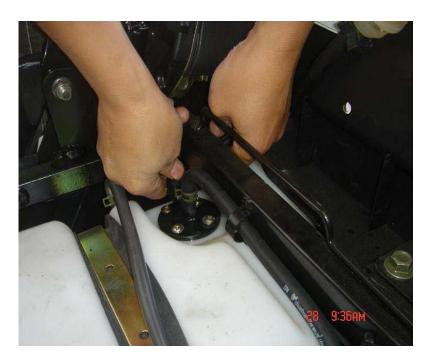
STEP 3: DISCONNECT THE HOSE FROM THE FUEL TANK. (IN THIS PICTURE IT IS THE HOSE IN THE BACK)
